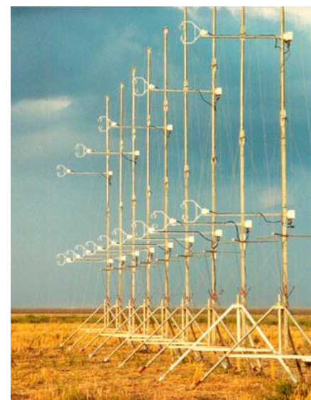
Figure 2: Sonic anemometer attached to pole. http://www.ucar.edu/communications/staffnotes/0412/awards.html
